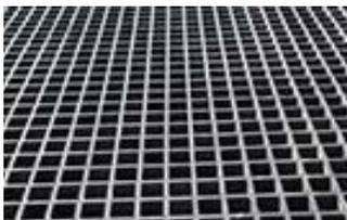
**Molded FRP Grating:** One piece construction. Standard panels; (1-2" thick) 3' x 10', 4' x 8', 4' x 12'. Mesh sizes; 1-1/2" square 1" x 4", and 2" square mesh. Standard colors are yellow, gray, green, and orange, with optional colors available. Fasteners available for all grating.
